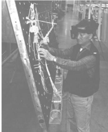
Figure 9 a) b). Aircraft manufacturing use of augmented reality
