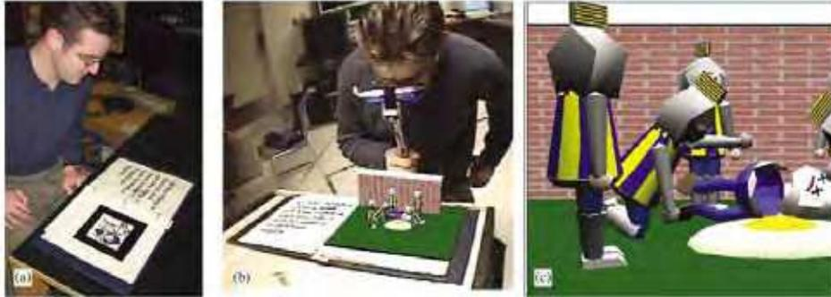
Figure 11. MagicBook with normal view (left), exo-centric view AR (middle), and immersed ego-centric view (right) (Billinghurst, Kato et al. 2001)
