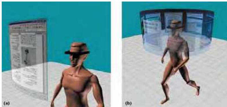
Figure 19. Head stabilised AR information display (left) and body stabilised (right) (Billinghurst, Bowskill et al. 1998)
