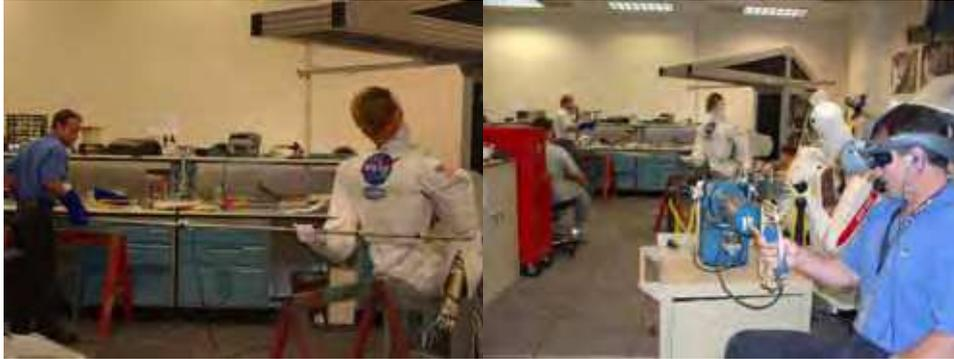
Figure 6. Robonaut working with a human (left) and human teleoperating Robonaut (right) (Glassmire, O'Malley et al. 2004)
